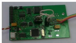
Prototype ARINC-429 to USB interface Electronics and software design
